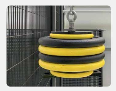
Mass release height from the ground (mass load center): h0 = 3,060 m Mass impact height from the ground (mass load center): h1 = 1,420 m  $\Delta H = h0 - h1 = 3,06 - 1,42 = 1,64$  m
